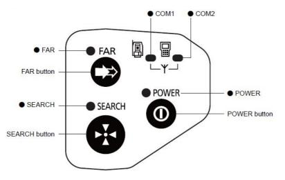
Press and hold the FAR button for about 10 seconds. When the beep sounds several times release
