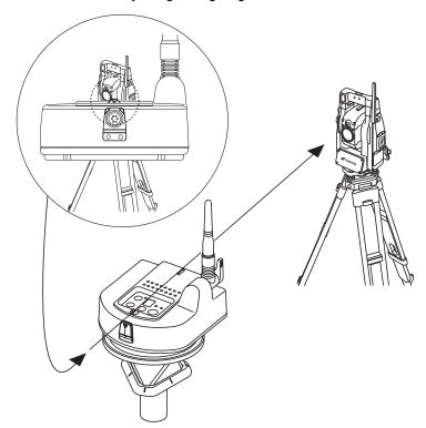
4 Press the [turn-round] key on the RC-4R. TS/IS/QS starts searching and ends in the tracking mode.
