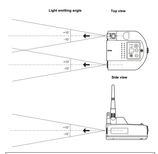
At greater distances, the laser light at the edge of the beam field (angle) will be weaker.
