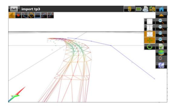
Allow users to select Multi-segment linework on the map and stake the intersection of two segments
