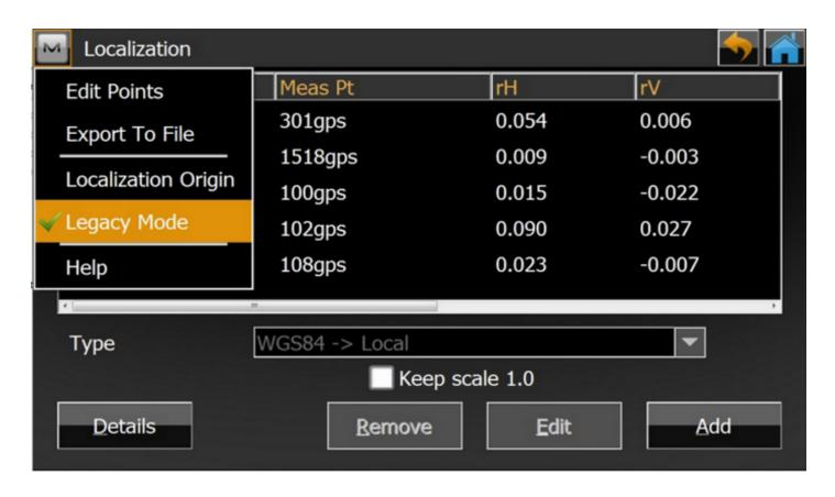
In addition to support for Legacy Mode, users can also choose the Localization Origin. The two options available are: Center of Localization Points and First Localization Point. The c ombinations available are described below.
