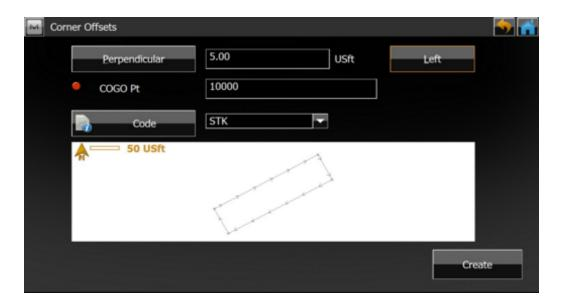
Enter Plan: Easily enter plan dimensions to create points and lines (optional).
