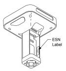
The ESN number can also be found by connecting the modem of the receiver to \*Topcon Receiver Utility (TRU) (version 2.2 or newer) and then selecting Settings tab Quick/Settings Info button. You can then retrieve the module S/N or ESN number.
